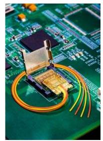
type of optical cable that it hopes will be fast, cheap, and thin enough to make it an attractive replacement for multiple copper wires.
